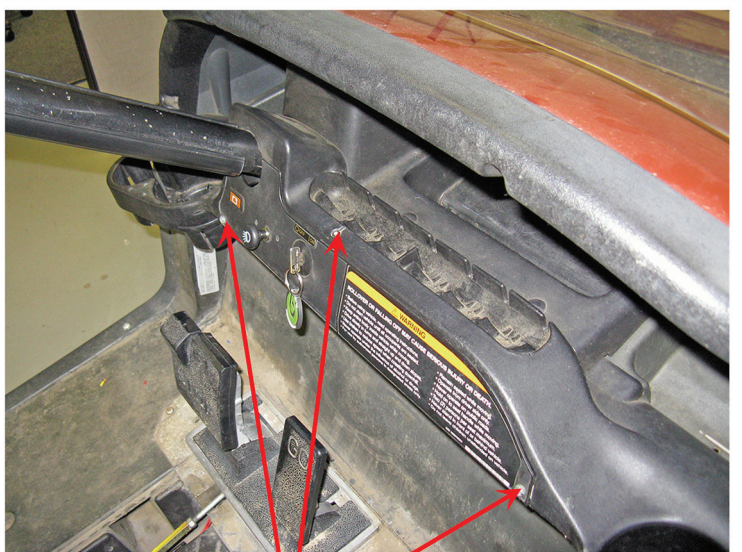
Remove Three Dash Screws
